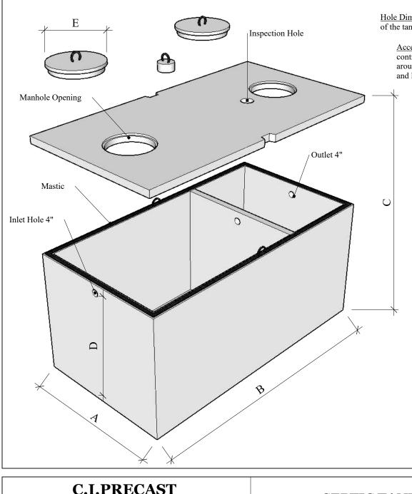
Hole Dimensions: The hole should be dug 2' wider and 2' longer than the external dimensions of the tank. The bottom should be leveled with 4" of graded material in the bottom.
